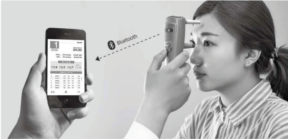
Bluetooth data transmission, 24 Hours IOP Monitoring, Display the Trend Chart of IOP Changing, provide effective support for the long-term monitoring of glaucoma.
